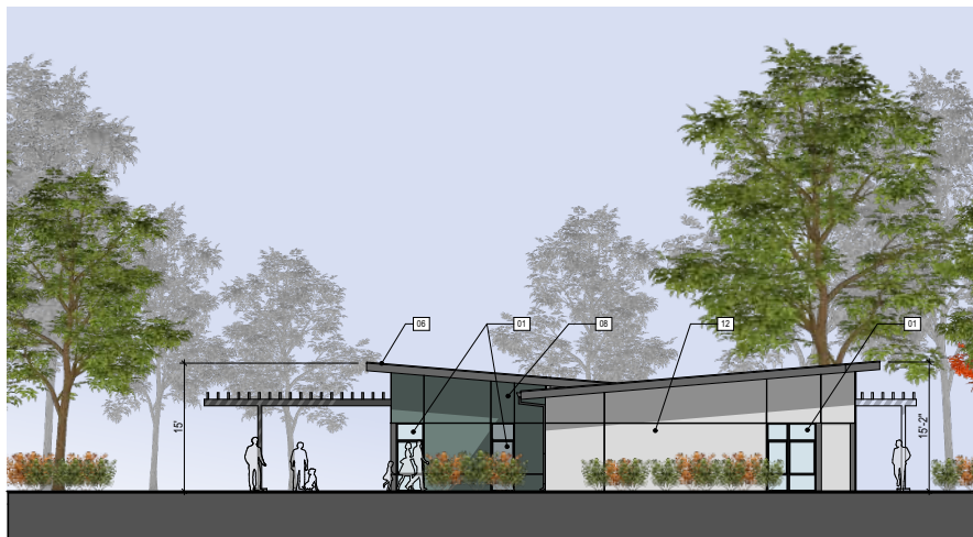
Community Building - Right Elevation - Scale 1/16" = 1'-0"
